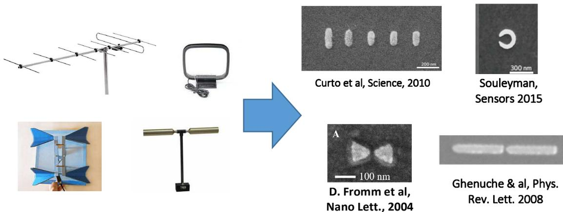
Figure 1: Four examples of antennas operating at radiofrequency and microwave regimes (left panel) and their optical counterparts (called nano-antennas) (right panel).
